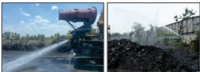
On-site field inspection of dust-suppression measures adopted by the project proponent to maintain air quality in Khairaha UG mines against the laid down standards
