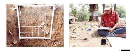
Measurement of unsaturated soil hydraulic conductivity using mini disk infiltrometer
