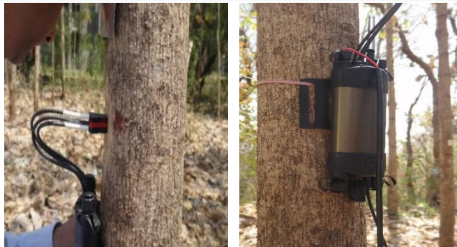
Installation of Sap flow instrument in Tectona grandis trees
