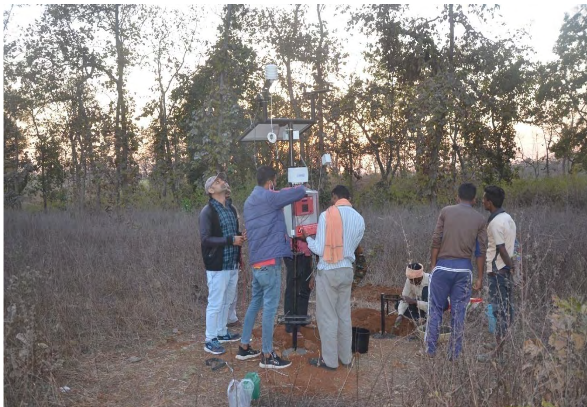
Fig. 38: Installation of AWS at Moiya Nala, West Mandla forest division
