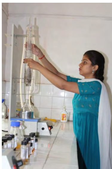
Fig. 40: Extraction of seed oil using Soxhlet Apparatus.
