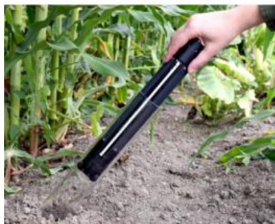
Field operation of a common minirhizotron with a wireless interface as advancement (Image Credits: Rahman et al. , 2020)
