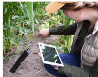
Field operation of a common minirhizotron with a wireless interface as advancement (Image Credits: Rahman et al. , 2020)
